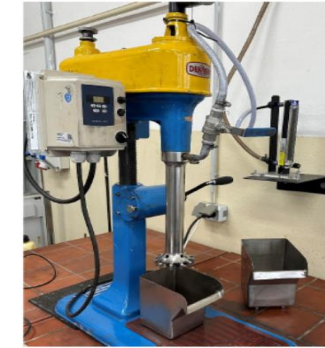
Fig: Single unit-operation for flotation at lab-scale
